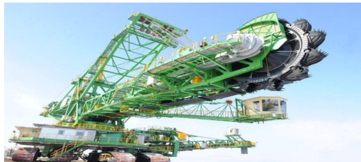
Bucket-wheel crawler excavator KWK 1500.1
