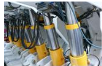
Hydraulic props (legs) covered with DURACHROM unique protective ecological coatings
